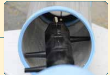
Self Suction Cleaning Mechanism Cleaning of filter is carried out by smart suction mechanism which rotates spirally across the screen
